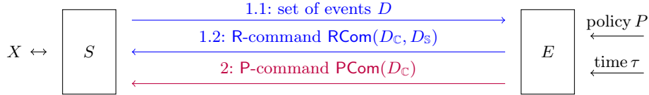
Fig. 2. System model for proactive real-time first-order enforcement
